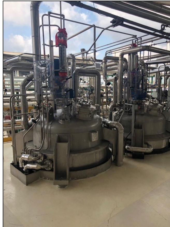
Images: Fermenter and Chromatographic purification at European CMO
